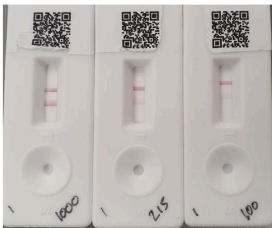
Fig. 8. Results from urinary 1-OHPyrG Lateral Flow Immunoassays. LF cassettes developed at three 1-OHPyrG concentrations (100–1000 pg/ml).
